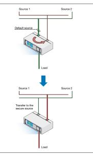
The detection of a failure in the preferred source triggers the automatic and instantaneous transfer to the alternate source without disturbing the supply to the load. The "break before make" transfer is carried out without overlapping in order to prevent interference between the sources.
